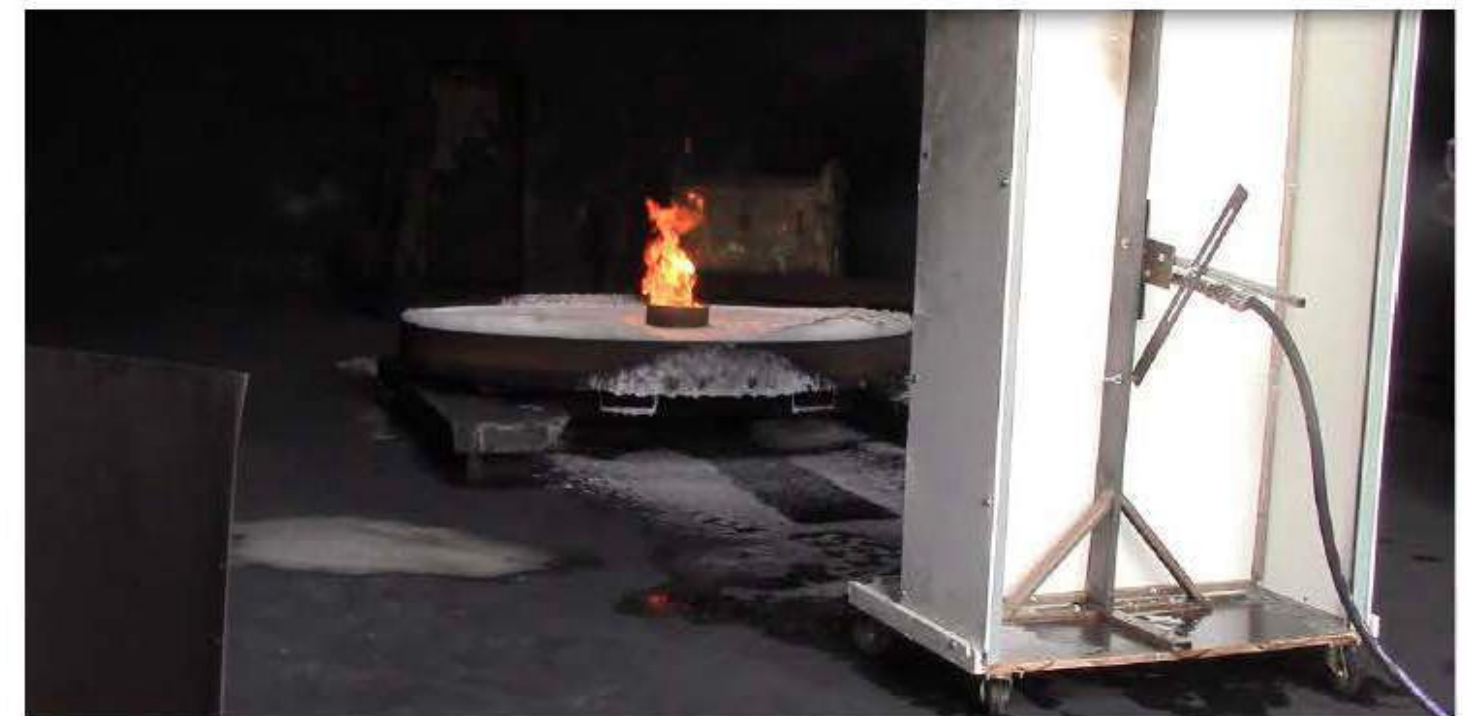
Photograph A4: burn-back test
